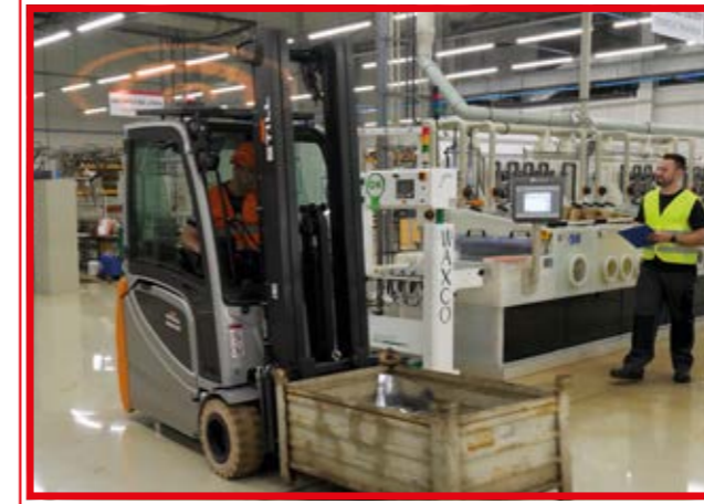
warning zone - forklift autonomously decelerates, personal tag vibrates
