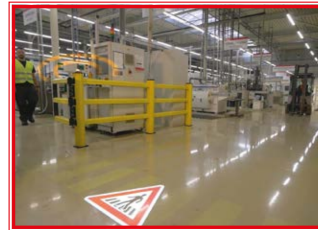
warning zone - connectivity to LED floor marking (symbol changing)
